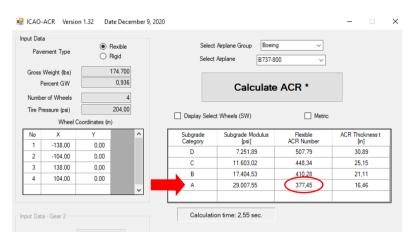
b) Obtain the PCR for the surface on which you are going to operate;
