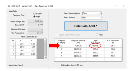
b) Obtain the PCR for the surface on which you are going to operate;
