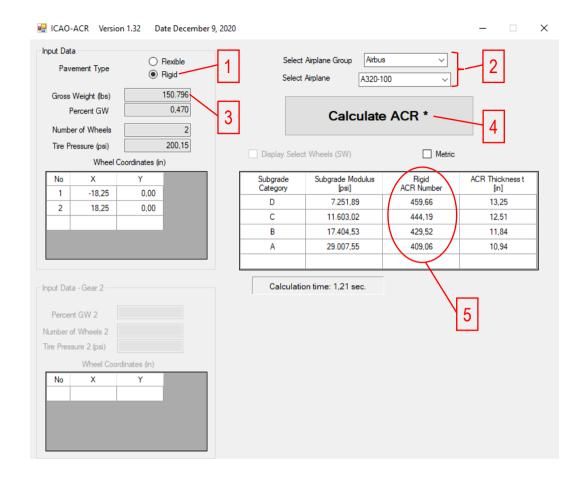
In our case, the value of the PCR = 480 / R / B / W / T, T, indicates that the strength category of the foundation soil is **B**, therefore, from the result, we must choose the ACR corresponding to the strength category of the soil of foundation **B**.
